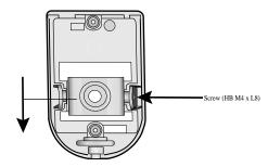
Assemble the assy-case front onto the case-rear as shown in the illustration. Fasten the assy-case front to the case-rear with the screw (BH M2.6) you removed earlier.
